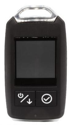
The AirID Mini is a wearable SIM-sized card reader in a keyfob style, with two buttons. The device acts as a robust housing for a SAM, a SIM-sized smartcard, that can be used as a key fob, removing the risk of FIDO tokens left in place. It transfers data securely over Bluetooth (BLE) or a USB connection.
